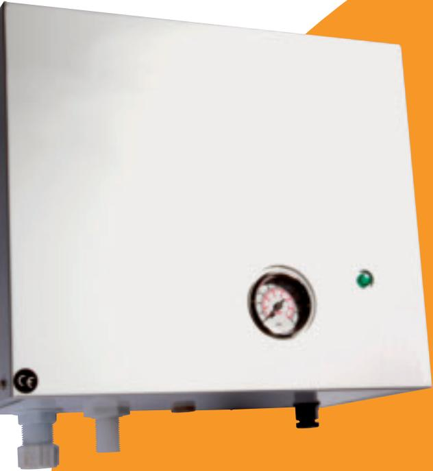
The Mini Pressurisation Unit is a compact wall mounted unit housing either one or two small pressurisation pumps and associated control equipment for connecting to small heating or cooling installations within large domestic dwellings or small industrial/commercial installations.
